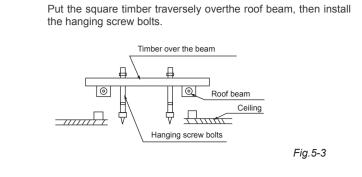
Do keep the ceiling flat. Consolidate the roof beam to avoid
